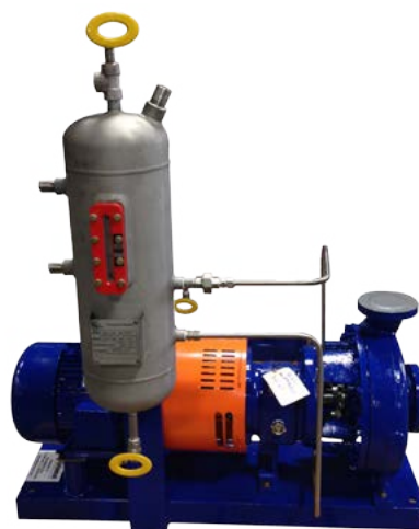
CPI PLAN 7353 Pressurized circulation lubricates double seal faces.
